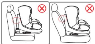
Push the car seat against the passenger seat, making sure that both ISOFIX connectors are extended in the same position. There must not be any space between the backrest of the passenger seat and the car seat.
