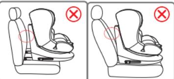
Push the car seat against the passenger seat, making sure that both ISOFIX connectors are extended in the same position. There must not be any space between the backrest of the passenger seat and the car seat.
