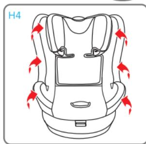
Carefully replace the lining along the edge of the headrest, in its housing. Attach the press studs on the headrest and seat fabric.
