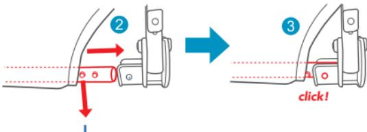
**IMPORTANT:** Make sure that the metal pin is correctly locked in its hole, a "click" will indicate that it has locked in successfully.
